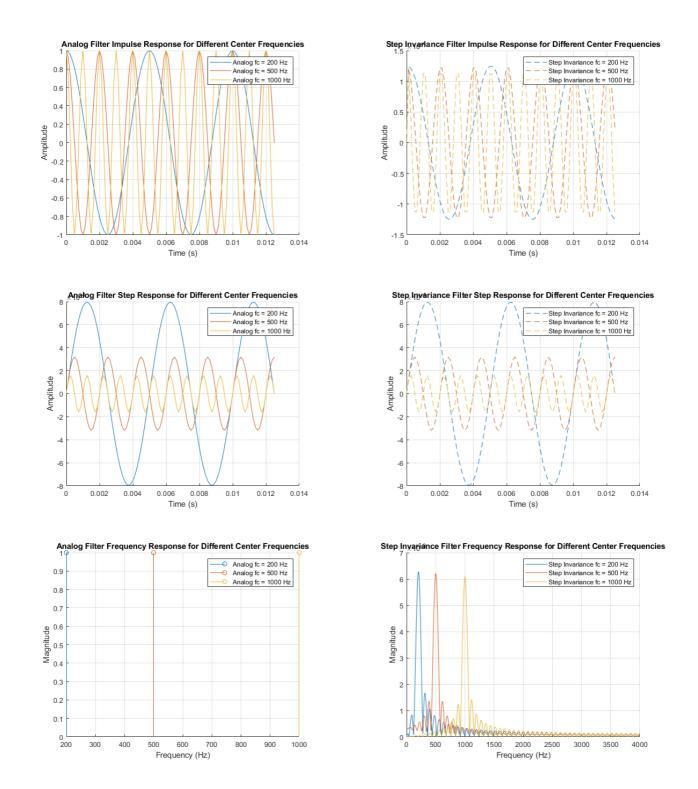
Step Response remains consistent after turning analog filter into IIR filter using step invariance method.
